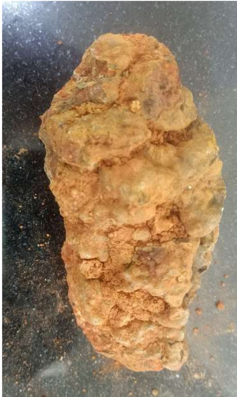
Photo 6: Laterite with botryoidal structure.
