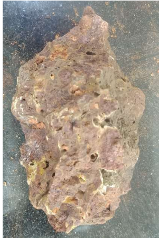
Photo 7: Laterite with pisolitic structure.
